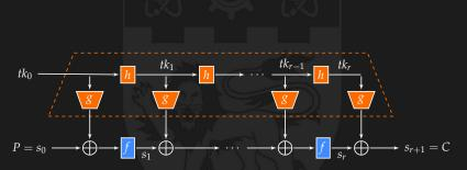
TWEAKEY generalizes the class of key-alternating ciphers
