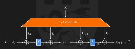
General construction of a block cipher : iterated block ciphers
