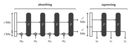
The (c + r)-bit internal state is viewed as a  $d \times d$  matrix of *s*-bit cells.
