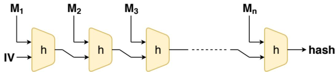
The compression function  $h$  now takes two fixed-size inputs, the incoming chaining variable  $CV_i$  and the message block  $M_i$ , and outputs a new chaining variable  $CV_{i+1}$ .
