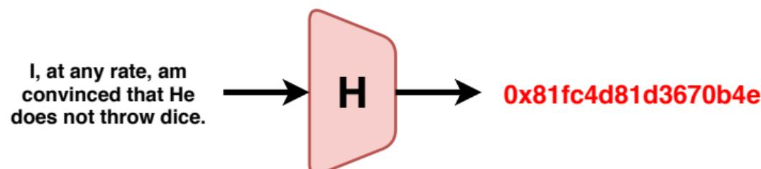
$H$  maps an **arbitrary length input** (the message  $M$ ) to a **fixed length  $n$ -bit output**.
