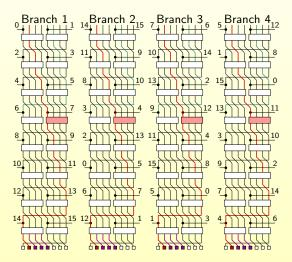
By introducing differences in  $B_0$  and finding simultaneous microcollisions in four Q-structures in step 4 we obtain a differential restricted to 4 registers.
