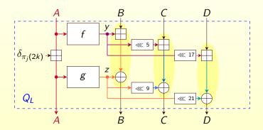
Micro-collision: a difference in register A does not propagate to the selected register B, C or D.
